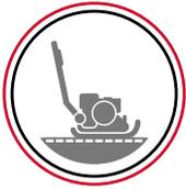
Use of a plate or roller compactor is recommended. If using a plate, a protective pad should be used to protect the paving surface.
